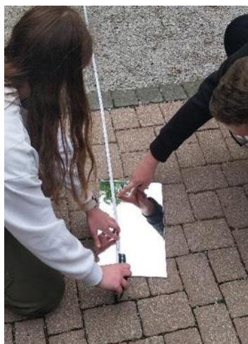
Figure 28 Measuring tree height using a mirror – triangle similarity
