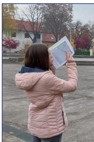
Figure 29 Measuring tree height using a clinometer
