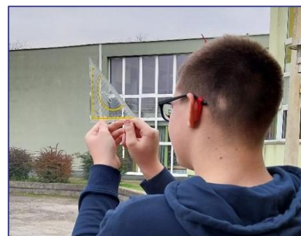
Figure 30 . Measuring tree height using an isosceles right triangle
